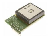
The selected module is one of the cheapest and simplest. Nevertheless, the manufacturer promises the presence of a battery for storing satellite data. An important parameter of devices connected to the Arduino – power consumption. If you overload the Arduino converter, it may burn. For the receiver used, the maximum power consumption is 45mA.
