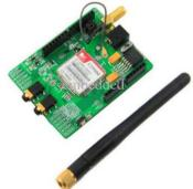
GSM module – SIM900. It supports GSM and GPRS. Neither EDGE, nor even 3G, are supported. This is probably good for transferring coordinate data – there will be no delays and problems when switching between modes, plus GPRS is almost everywhere now.
